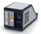
The D140 measures the distance between the laser and the receiver. Use the excentric screw to align the laser horizontally or vertically. There is an automated bluetooth communication between the D140 and the ProLine® software. It is possible to measure fully automatically. Furthermore the possibility for incorrect measurements is minimized.
