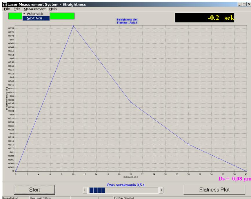
FIG.7.4. CHANGING AXIS IN FLATNESS MEASUREMENT
