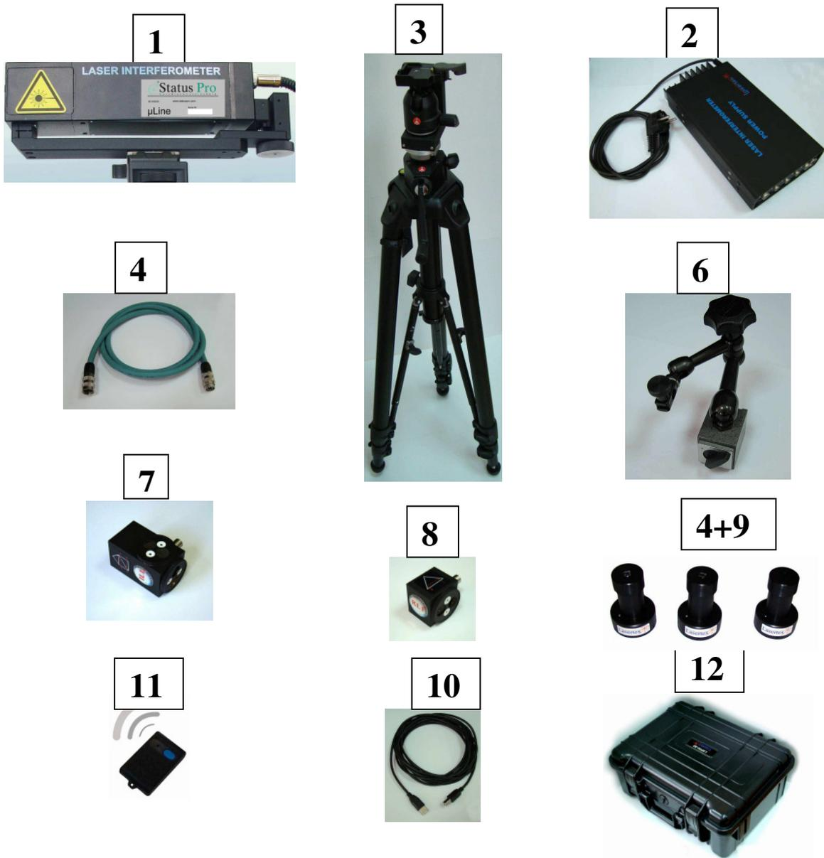
FIG.3.1b. THE ELEMENTS OF THE STANDARD SET
