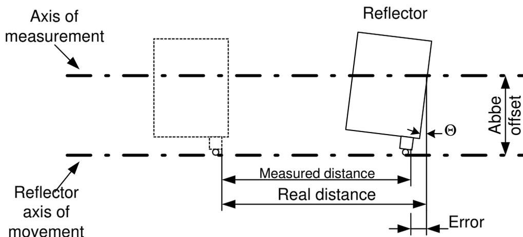
**FIG.2.6. AN ILLUSTRATION OF AN ABBE ERROR**
