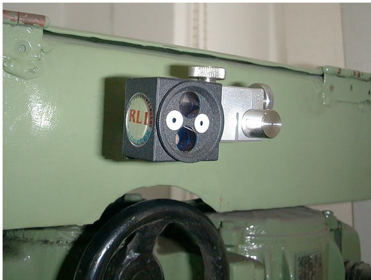
FIG.8.2. EXAMPLE OF PROPERLY ATTACHED RETRO-REFLECTOR
