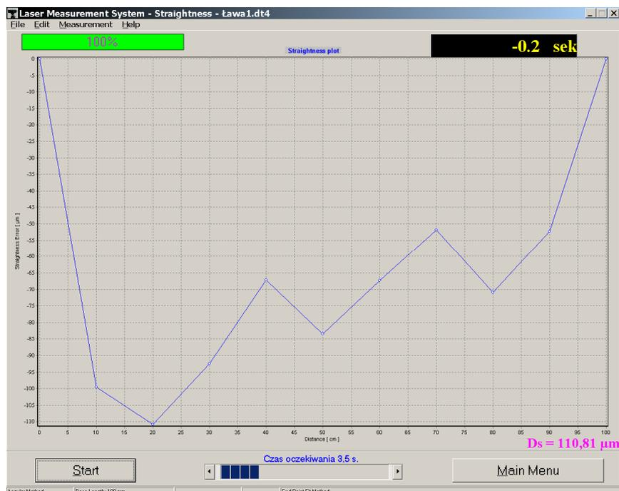
FIG.6.6. A RESULT OF STREIGHTNESS MEASUREMENT
