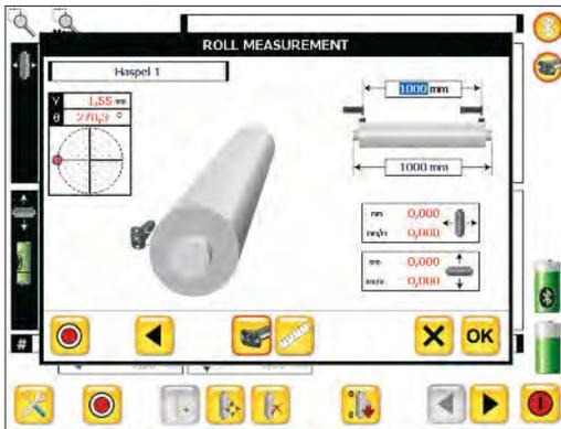
Position your sensor. The sensor has a inclinometer in it so it "knows" the angle. The current angle and measurement value is displayed top left. Press "Measure".
