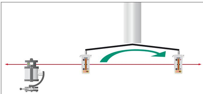
Using the reference plane of the T310 and a sensor arm, fix the R310 to an arm. Attach the arm to the roll stub. Now rotate the roll. This is a very easy way to measure the vertical and horizontal angular deviation with respect to the reference plane. This method is used often for hidden rolls or wheels.
