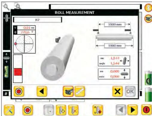
The sensor symbol will jump to the other end of the roll. Position your sensor there. The red bar meter will ensure that you are at the same angle as the first measurement. When you are positioned correctly press "Measure".
