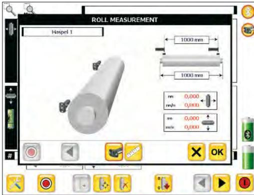
This is the measurement screen. Enter the roll length and the measurement length (if they differ). Touch the sensor symbol where you want to measure first.
